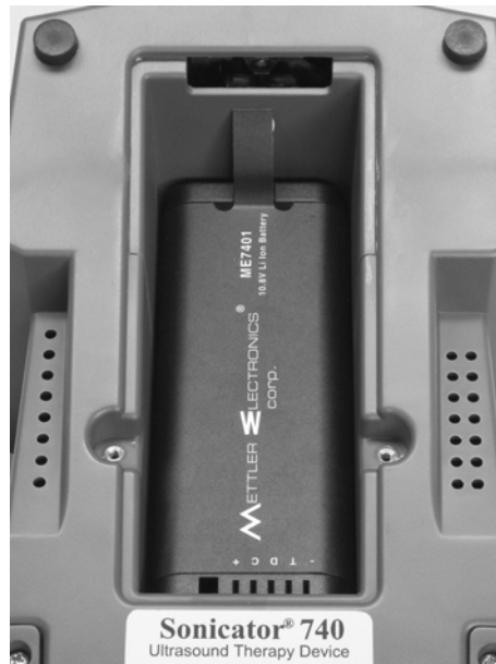
Figure 4.5—Installing the Battery
