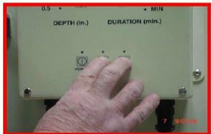
Press and Hold Start and Stop Buttons Until The Light Stops Flashing
