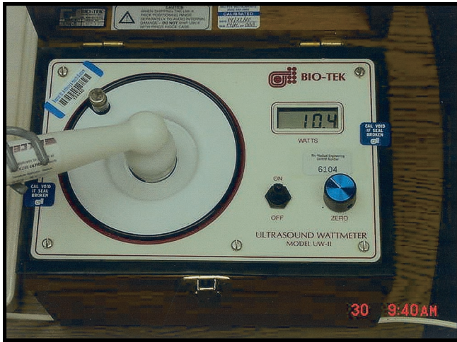
Figure 1. Illustration of Bio-Tek Digital Ultrasound Wattmeter (model UW-2) used to test power output.
